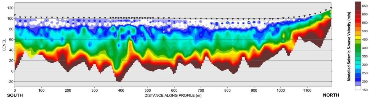
**Figure 4: Generated S-wave velocity section, showing the Vs model with level and distance. Depth is to ~100m and distance along the profile is 1200m. Vs values are shown as per the colour scale**
