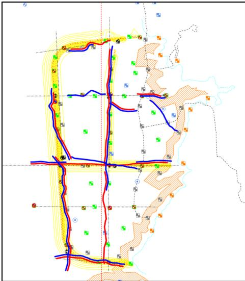
**Figure 1: Survey area and lines of ReMi over the proposed TSF. Red lines indicate Deep ReMi, Blue lines indicate Shallow ReMi data collection.**
