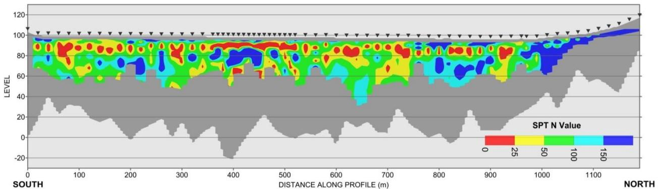
**Figure 6: Modelled SPT value generated with correlation to the ReMi S-wave velocity sections.**
