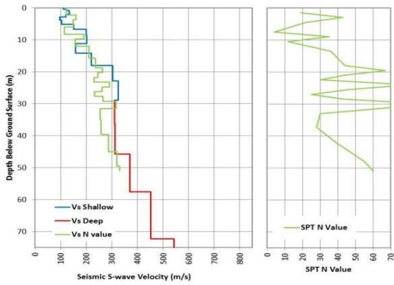
**Figure 3: Vs sounding for deep ReMi (red), shallow ReMi (blue) and converted SPT values (green).**
