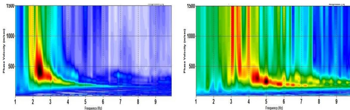
**Figure 2: Generated dispersion curves for the deep ReMi setup (left) and shallow ReMi set up (right)**
